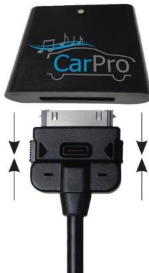
1. Locate the 30-Pin iPod connector that comes with the original iPod integration.
